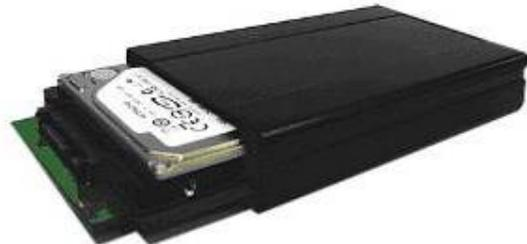
4. Carefully replace the two screws to secure the removable caddy end. Do NOT over tighten the screws.
